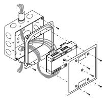
**SIGA-MCC1S:** mount the UIOxR motherboard inside a suitable GE Security enclosure with screws and washers provided. Plug the module into any available position on the motherboard and secure the module to the motherboard with the captive screws. Wiring connections are made to the terminals on the motherboard (see wiring diagram). UIOxR motherboard terminals are suited for #12 to #18 AWG (2.5 mm<sup>2</sup> to 0.75 mm<sup>2</sup>) wire size.
